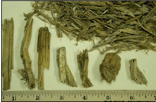
Figure 1. Rind pieces in mill-run bagasse (scale in inches).
