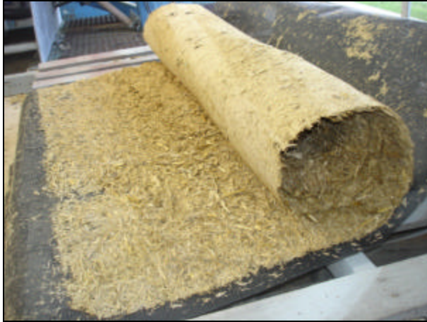
Figure 6. A partially rolled and dried bagasse mat.
