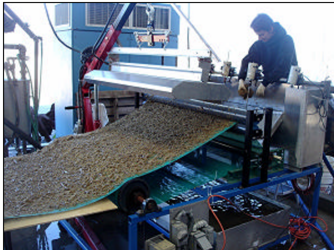
Figure 5. The mat formation process: bagasse fibers are added manually into the feed tank and the bagasse slurry overflows onto the moving mesh belt forming the mat.
